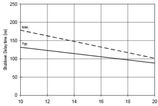
Figure 9B. Shutdown Time vs. Vcc/Vbs Supply Voltage
