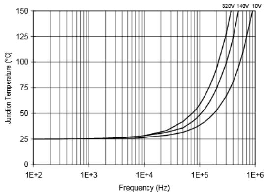
**Figure 35. IR2110S/IR2113S  $T_J$  vs. Frequency**
