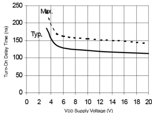
**Figure 7C. Turn-On Time vs. VDD Supply Voltage**
