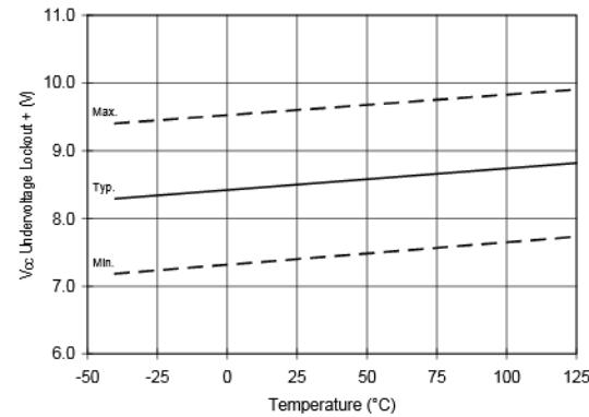
Figure 24.  $V_{CC}$  Undervoltage Lockout (+) vs. Temperature
