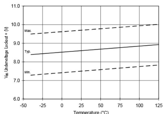
Figure 22.  $V_{BS}$  Undervoltage Lockout (+) vs. Temperature
