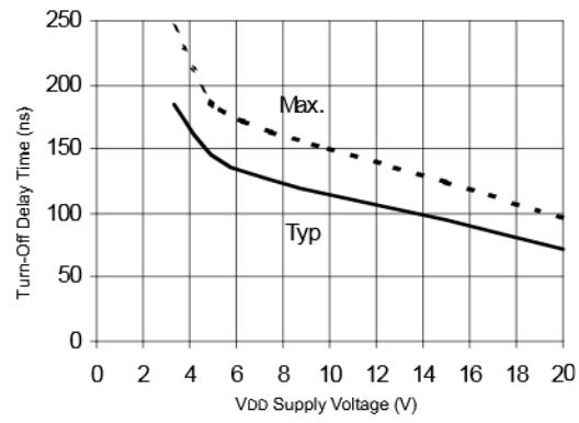
**Figure 8C. Turn-Off Time vs. Vdd Supply Voltage**
