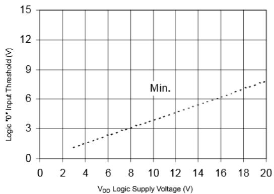
Figure 13B. Logic "0" Input Threshold vs. Voltage
