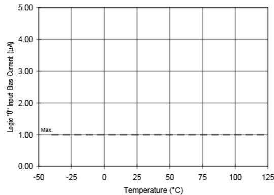
Figure 21A. Logic "0" Input Current vs. Temperature
