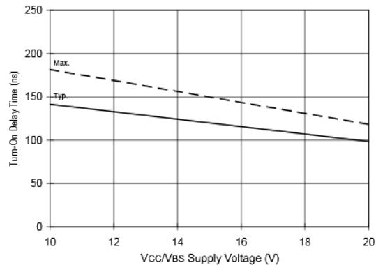
**Figure 7B. Turn-On Time vs. Vcc/Vbs Supply Voltage**
