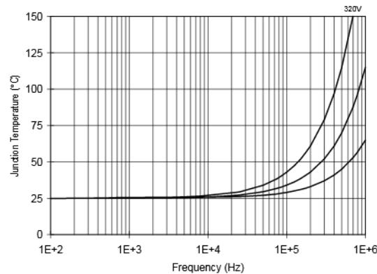
**Figure 29. IR2110/IT2113  $T_J$  vs. Frequency**
